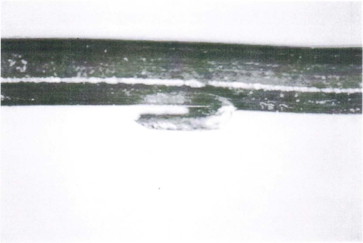
Fig.2. Copper wire defects. Defect sizes are about 2.5 mm.
